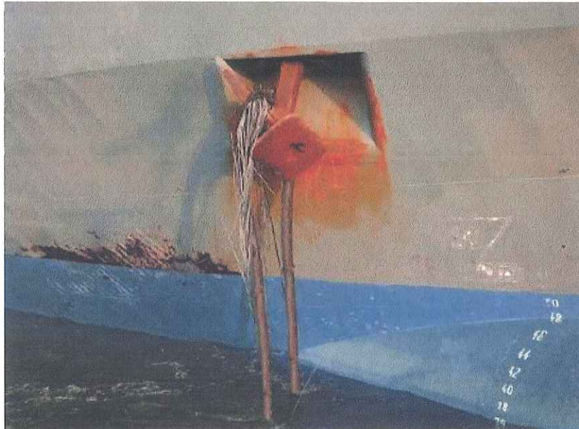
Figure 4-1 Vessel's anchor fouled a power cable
